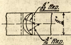
Fig. 48a.—Enlarged Drawing of Blades. (Plan.)
