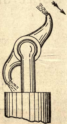
Fig. 2.—Hero's Reaction Engine.
