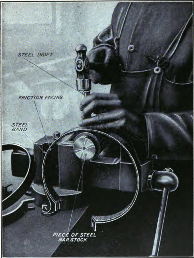
Fig. 92.—How Friction Lining is Riveted to Brake Bands.
