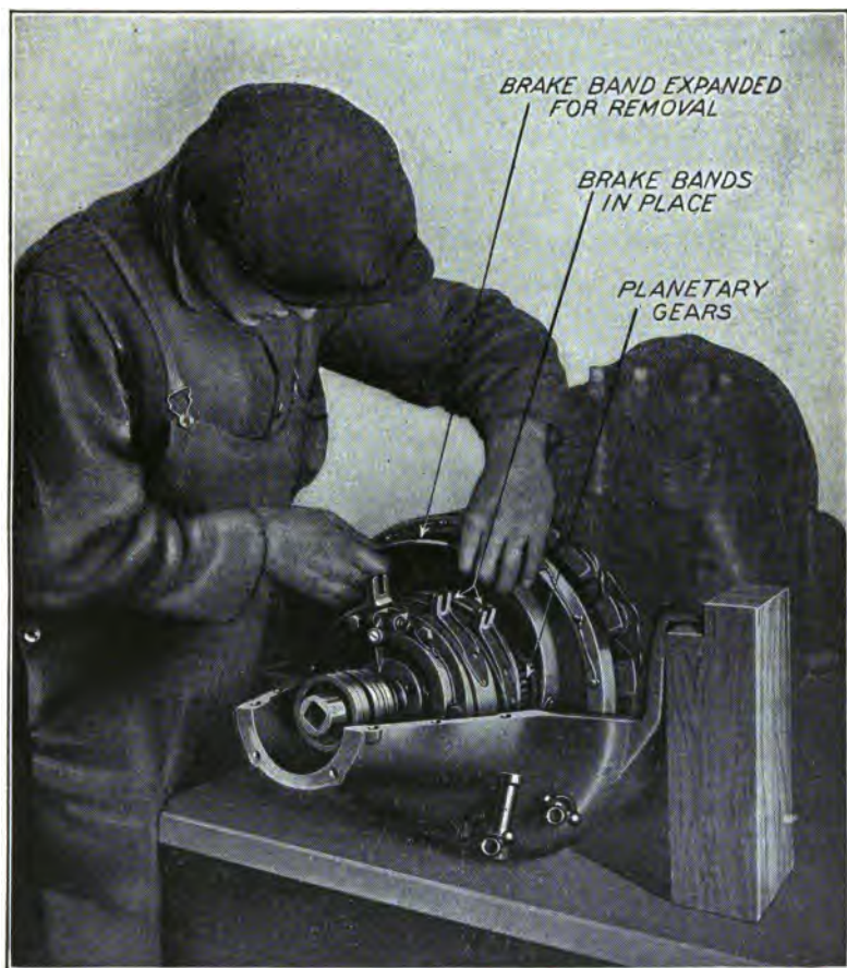
Fig. 91.—Removing Transmission Brake Band for Replacing Friction Lining.
