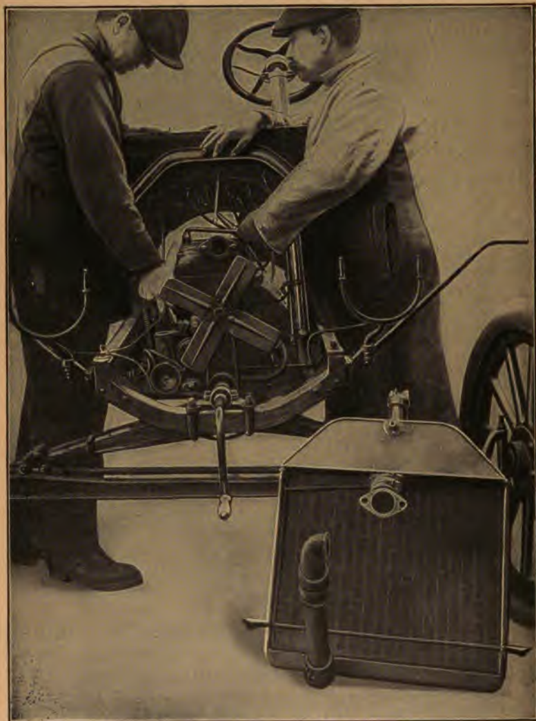
Fig. 68.—The First Step in Removing the Ford Engine From the Chassis Is to Take the Radiator From the Front of the Frame.
