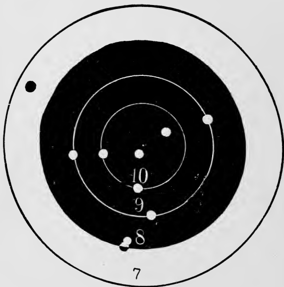
Score of 90 out of a possible 100, at 30 yards, with gallery ammunition, in .44 calibre Smith & Wesson Russian-model revolver, made by Mr. F. E. BENNETT, at Walnut Hill, Mass., Oct. 12, 1887. Reduced one-half.
