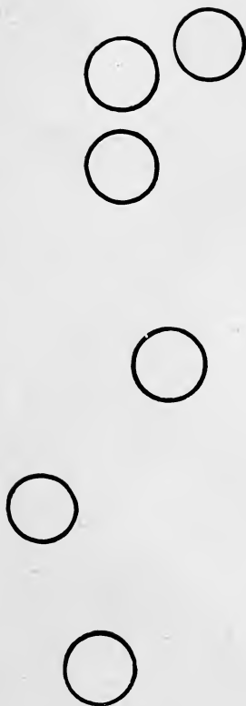
Diagram of six consecutive shots, fired from a rest, at 50 yards, with a Colt's Frontier Model revolver, .44 calibre, full charge, — 40 grains of powder, 200 grains of lead.
