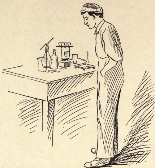
FIG. 27—Parting porcelain capsules in sand bath over small kerosene stove.
