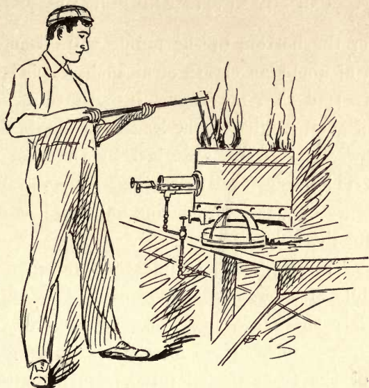
FIG. 63—Stirring molten bullion with graphite stirring rod.
