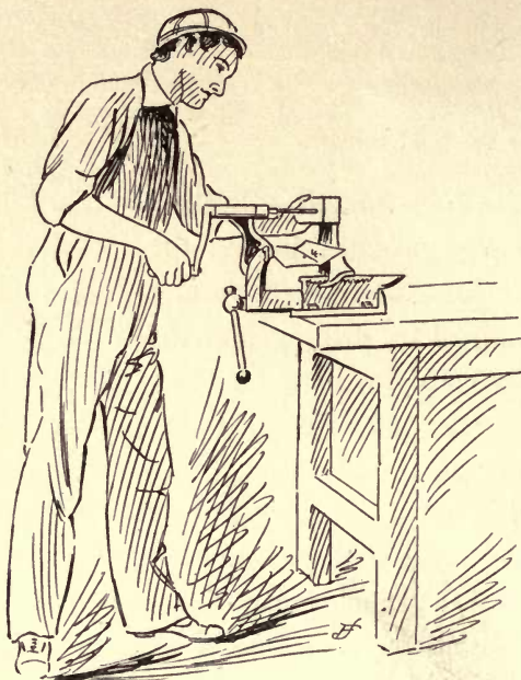
FIG. 32—Drilling out sample of bullion brick.
