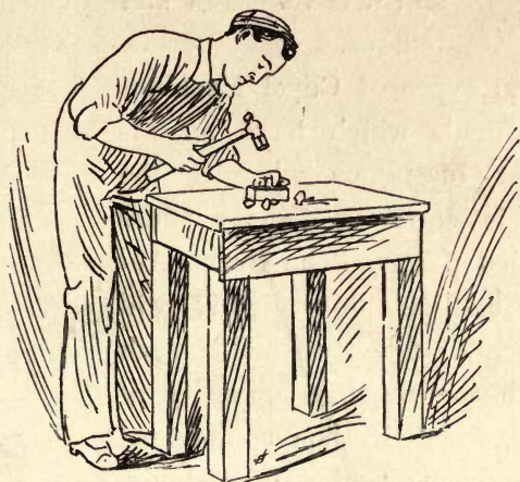
FIG. 14—Breaking slag away from lead button.
