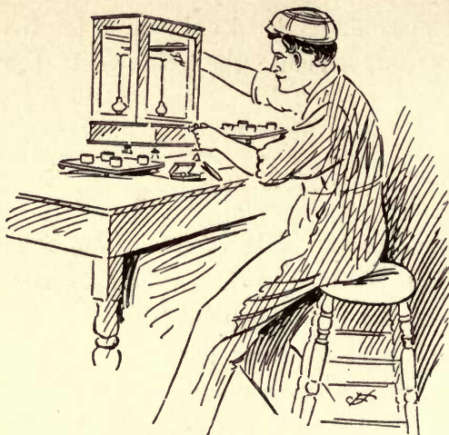
FIG. 23—Weighing bead on button balance.
