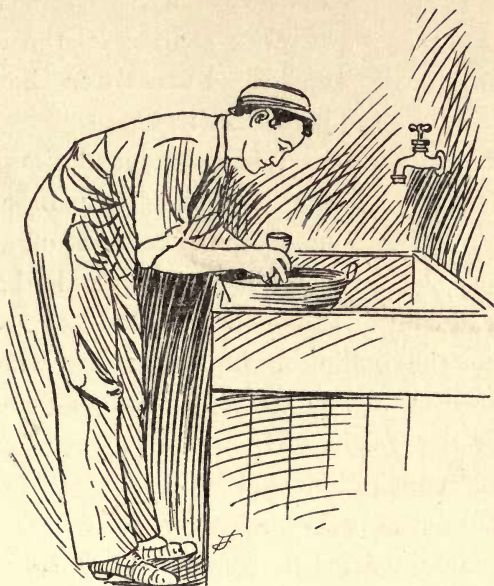
FIG. 39—Transferring coronet from flask to annealing cup under water.
