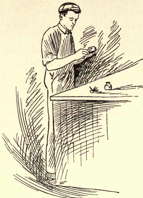
FIG. 48—Testing gold fineness with test needles and touch stones.
