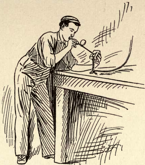
FIG. 25—Fusing assay bead and silver foil, called "quartation."
