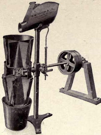
FIG. 3a—Umpire Automatic Ore Sampler, power (sectional view).
