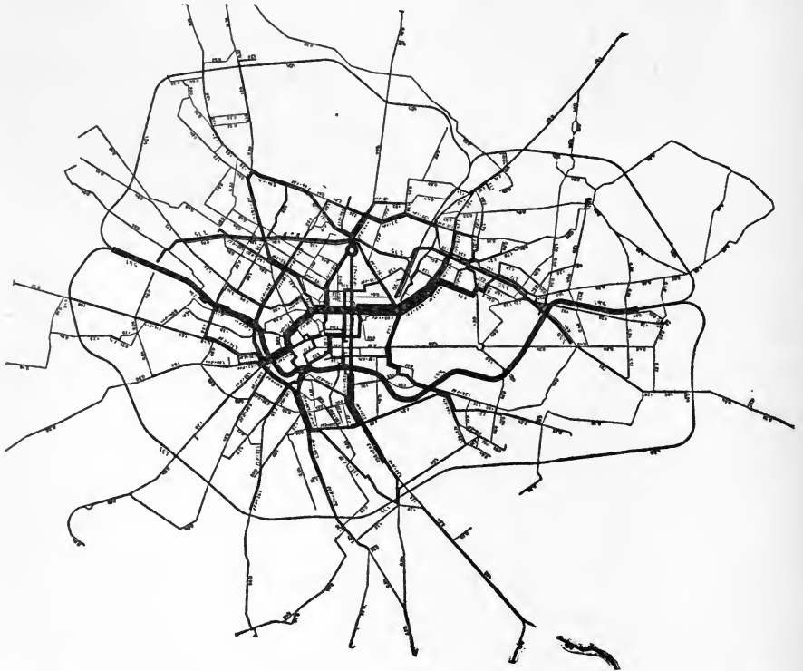
FIG. 29. VOLUME OF TRAFFIC IN BERLIN, INCLUDING CITY AND BELT RAILWAYS, ELEVATED AND SUBWAY, SURFACE CAR AND OMNIBUS LINES
