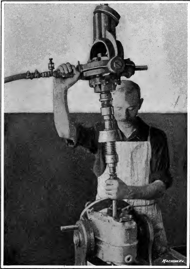
Fig. 14. Pneumatic Drill screwing in Cap-screws
