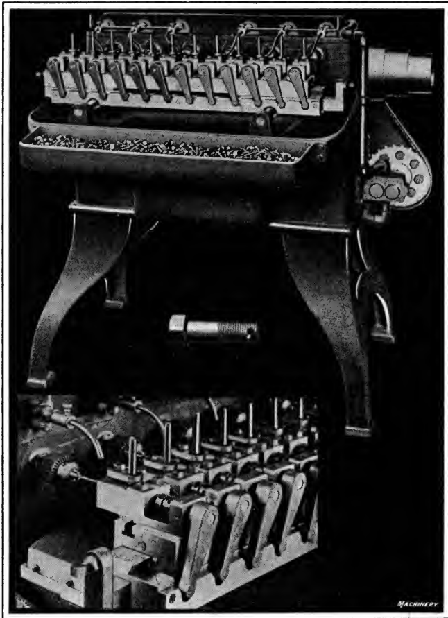
Fig. 3. Six-spindle Semi-automatic Drilling Machine with Double Work-holding Fixture which provides for Loading Six Sections of Fixture while Work is being drilled in Other Six Positions
