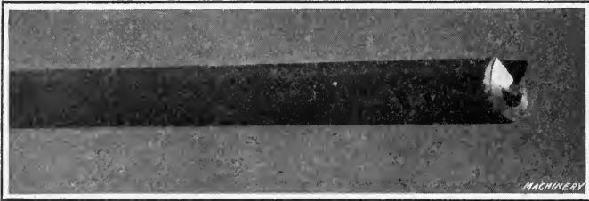
Fig. 11. Cutting End of a Rifle Barrel Drill
