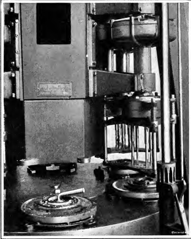
Fig. 17. View of Loading Station of Drilling Machine shown in Fig. 16
