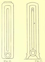
Intermediate and End Sections of Radiator Shown in Fig. 15. The end sections (at right) have legs.
