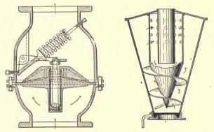
Fig. 117. Back-Pressure Valve Automatically Operated by a Spring.
