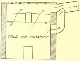
Fig. 61. Heater and Mixing Damper with Brick Casing. Damper between Heater and Register.
