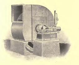
Fig. 145. Centrifugal Fan in "Three-Quarter Housing." Used where Headroom is Limited; Extra Space Provided by Pit under Floor-Level.
