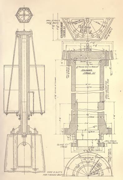
HYDRAULIC ACCUMULATOR Assembled Drawing with Details on the Same Sheet
