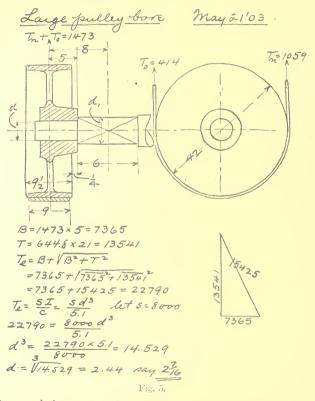
done partly because it is desired to show the student that the shaft at each of these points should be theoretically of different size. It is also done because as a practical feature of construction it is a good plan to change the size when the fit changes, partly for reasons of production in the shop, partly for ease in slipping pieces
