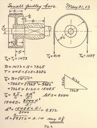
a long lapse of time. If the machine should unexpectedly fail in service the figures are always available to prove or disprove theoretical weakness. The right triangles merely indicate that the value of  $\sqrt{B^2 + T^2}$  was found by the graphical method suggested in
