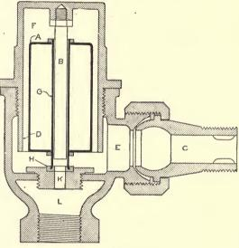
Fig. 131. Water-Seal Motor.
