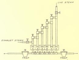
Fig. 140. Heater Made Up of Interchangeable Sections.
