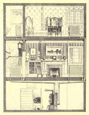
HOT WATER HEATER AND CONNECTIONS.
