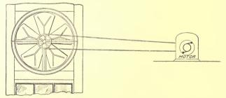
Fig. 151. Fan Belt-Connected to Motor.
