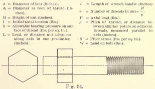
ANALYSIS. A bolt is simply a cylindrical bar of metal upset at one end to form a head, and having a thread at the other end, Fig. 54. A stud is a bolt in which the head is replaced by a thread; or it is a cylindrical bar threaded at both ends, usually
