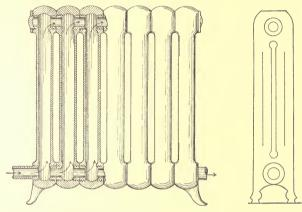
Fig. 86. Common Form of Hot-Water Radiator. Circulation Produced Wholly through Action of Gravity, Hot Water Rising to Top.
