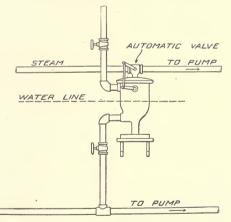
Fig. 121. Pump Regulator Placed at Sufficient Height to Raise Water-Line to Point Desired.
