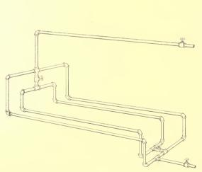
Fig. 177. Connections of Inner Groups of Pipes of Greenhouse Shown in Fig. 175.
