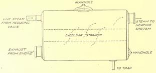
Fig. 115. Oil Separator Consisting of a Tank in which Steam is Filtered by Passing Upward through a Layer of Excelsior.
