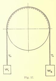
as in Fig. 17, the strap by its friction on the pulley will turn the pulley, and the force of friction F becomes the driving force for the pulley as noted in equation 5 above.
