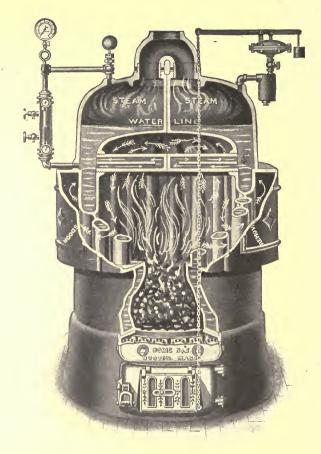
Cast Iron Seamless Tubular Steam Heater.
