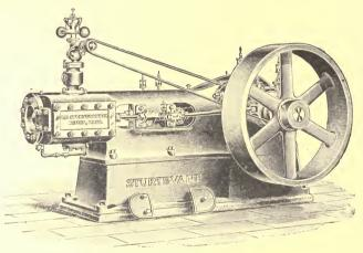
Fig. 154. Horizontal Engine for Fan Use.
