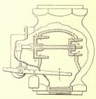
Fig. 116. Automatically Acting Back-Pressure Valve Attached to Vertical Pipe. For Preventing Rise of Pressure in System above any Desired Point.
