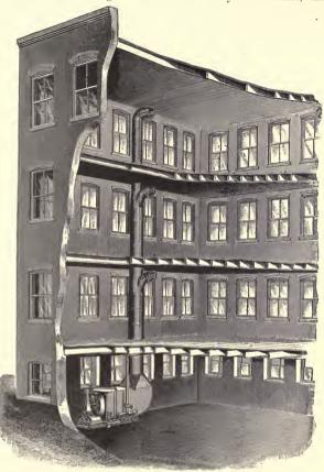
Fig. 158. Illustrating Application of Forced Blast for Warming a Factory.
