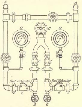
Fig. 134. Details of Connections at Exhauster, Paul System.
