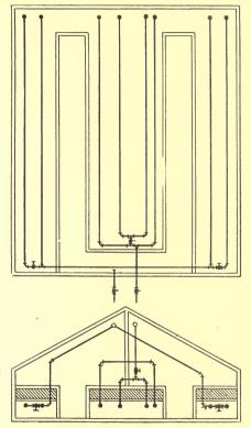
Fig. 175. Plan and Elevation Showing One Method of Running Piping in a Greenhouse
