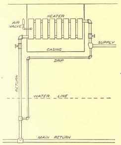
Fig. 75. General Method of Making Pipe and Radiator Connections, in Basement, in In lirect Heating.
