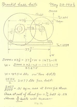
**carrying the load down to the base bolts, and the top serving as a tie between the bearings.**
