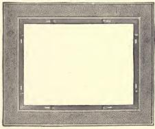
Fig. 71. Cast-Iron Border for a Floor Register.
