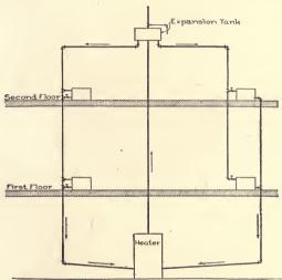
Fig. 90. "Overhead" Distribution System of Hot-Water Piping.
