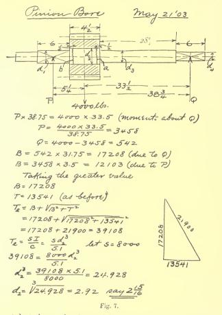
ported at the two bearings and having the tooth load applied as shown. If this latter effect be greater than the former, that is, if
