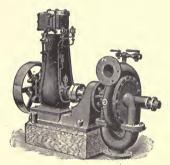
Fig. 111. Centrifugal Pump Direct-Connected to Engine, for Forced Hot-Water Circulation.
