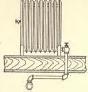
Fig. 30. "Two-Pipe" Connection of Radiator to Riser and Return.
