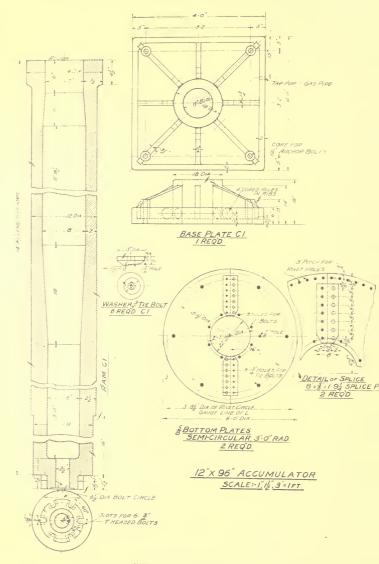
HYDRAULIC ACCUMULATOR Detail Drawing, to be used with Figure on Opposite Page
