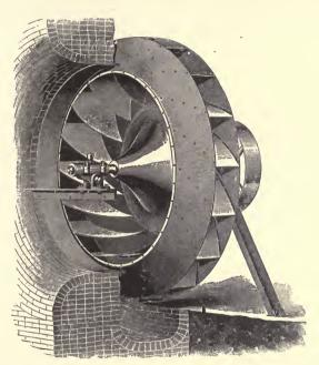
Flg. 146. "Cone" Fan. Discharges through Opening in Wall into a "Plenum Chamber" Connecting with Distributing Ducts.
