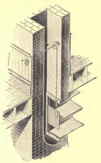
so that the air shall be forced, rather than drawn through the heater, and by providing a by-pass through which it may be discharged without passing across the heated pipes.
