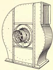
Fig. 143. Centrifugal Fan with Casing.
