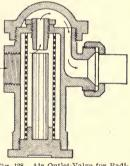
Fig. 128, Air Outlet-Valve for Radiator, Automatically Operated by Expansion and Contraction of Vulcanite Stem.
