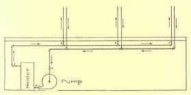
Fig. 109. "Two-Pipe" System for Forced Hot-Water Circulation.
