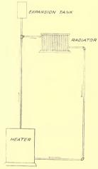
Fig. 84. Illustrating Simple Circulation in a Heating System.
