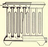
Fig. 85. Showing Construction of Radiator for Hot Water or Steam. Note Horizontal Passage along Top.
