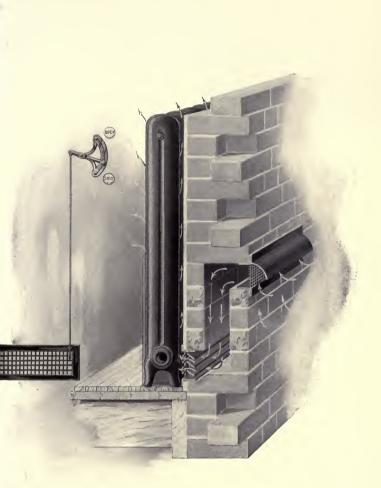
DIRECT-INDIRECT SYSTEM OF WARMING, SHOWING ADJUSTABLE DAMPER. American Radiator Company.
