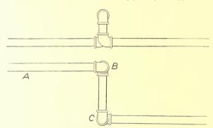
Fig. 33. Elevation and Plan of Swivel-Joint to Counteract Effects of Expansion and Contraction in Pipes.
