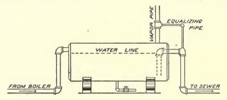
Fig. 49. Connections of Blow-Off Tank.
