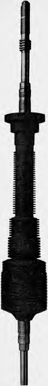
FIG. 22.—Rotor of Brush Company's Turbine.
