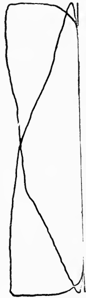
Low-Pressure Steam Cylinder. Scale \frac{1}{10} .
