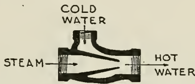
FIG. 25—McDANIEL'S SUCTION T, FROM WHICH COLD WATER, STEAM OR HOT WATER MAY BE DRAWN
