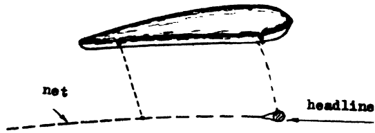
Fig. 4. Position of the plastic kite on the headline.
