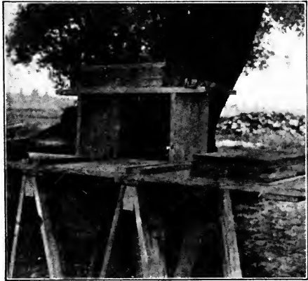
Fig. 33.—A FORM FOR SETTING UP APPLE BOXES
