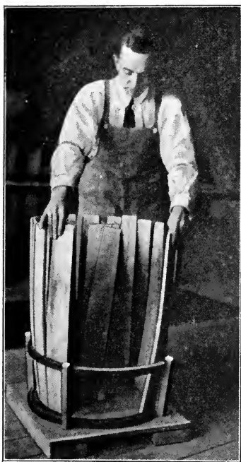
Fig. 38.—FORM FOR SETTING UP A BARREL
