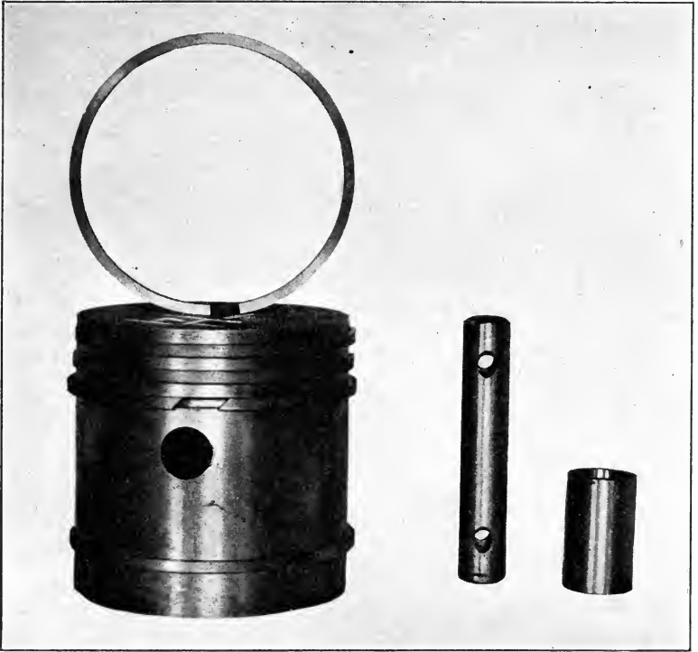
Fig. 98. —Showing Flat-Top Piston Provided with Four Concentric Rings, One of the Packing Members and the Wrist Pin with its Bushing.
