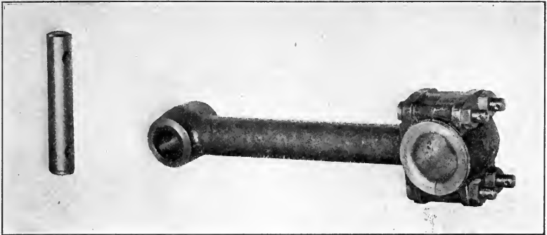
Fig. 99. —Typical Connecting Rod and its Wrist Pin. Lower Bearing Cap Held by Four Bolts. White Metal Boxes in Cast Bronze Rod.
