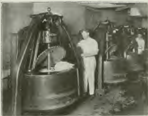
Fig. 3—Large Over-driven Extractors.
