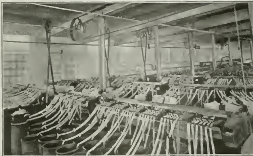
This section of the ending room of the Red Cross Cotton Mills gives a good idea of how the cotton ropes look as they come from the machines.
