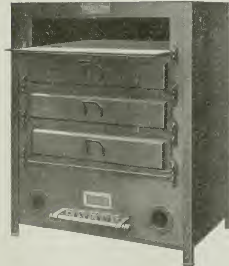
This cabinet bake oven has a capacity of ninety-six one-pound loaves of bread. It has four decks, each one lined with fire tile, and the bottom one doubly insulated and provided with bar gas burners for heating. Each deck has a separate door so that the contents of the deck may be inspected without disturbing all. The body of the oven is made of two thicknesses of sheet steel insulated with two inches of mineral wool.
