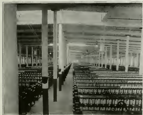
There are four different classes of machines through which the thread must pass in the spinning of yarn for gauze. In every stage the twisting is also going on. In this manner a rough rope an inch in diameter is transformed into a tightly spun fine thread.
