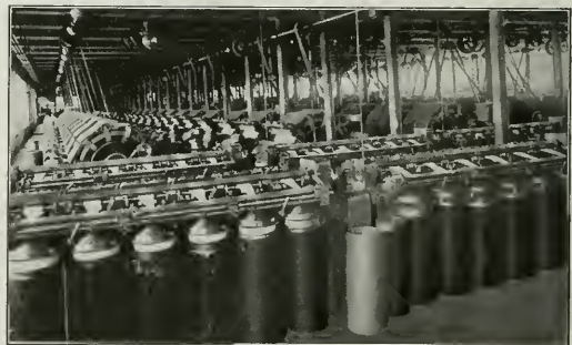
The heating and cleansing of cotton for the manufacture of surgical gauze is very much like that for the production of absorbent cotton, the main difference being that when the sheet emerges from the carding machine if it is intended for gauze, it is coiled into a loose rope called a "sliver." The picture shows a section of the carding room at the Chicopee Mills, Chicopee Falls, Mass.
