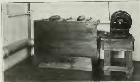
Rotary blower and air filtering box. The box contains two screened frames about eighteen by thirty-six inches, placed in its center. Between the frames is a layer of cotton. The air from the blower enters above the cotton and the outlet is below.
