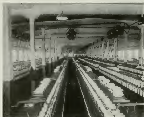
Spinning yarn for gauze is the reducing by gradual stages of the sliver or rope of fiber, turned out by the carding machines. This reduction is accomplished by stretching out, or attenuating, while at the same time the rope is made finer and stronger by twisting.
