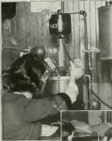
giving it a thin coating of wax. A dividing machine, adjusted to produce a fine or coarse scale as may be necessary in each individual tube, graduates the scale. The numbering of the degrees follows. During these processes the film of wax remains on the tube. It is now ready for the etching process. Hydrofluoric acid applied to the stem etches the glass where the wax has been cut away in graduating and numbering, to such a depth that when the wax is removed from the tube the lines and figures are deep enough to hold the indelible filling which makes them legible.
