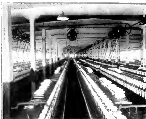
Spinning yarn for gauze is the reducing by gradual stages of the silver or rope of fiber, turned out by the carding machines. This reduction is accomplished by stretching out, or attenuating, while at the same time the rope is made finer and stronger by twisting.
