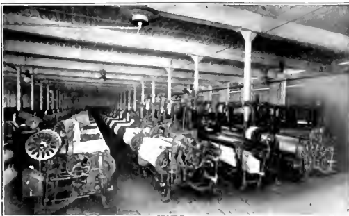
Weaving gauze in one of the weaving rooms at the Red Cross Cotton Mills. This method is slightly different from the old hand process when the weaver had to lift up every thread of the lengthwise threads and pass it under a shuttle containing the transverse thread.
