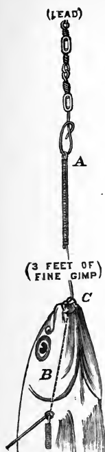
ATTACHMENT OF SPINNING BAIT WITHOUT LIP-HOOK.
