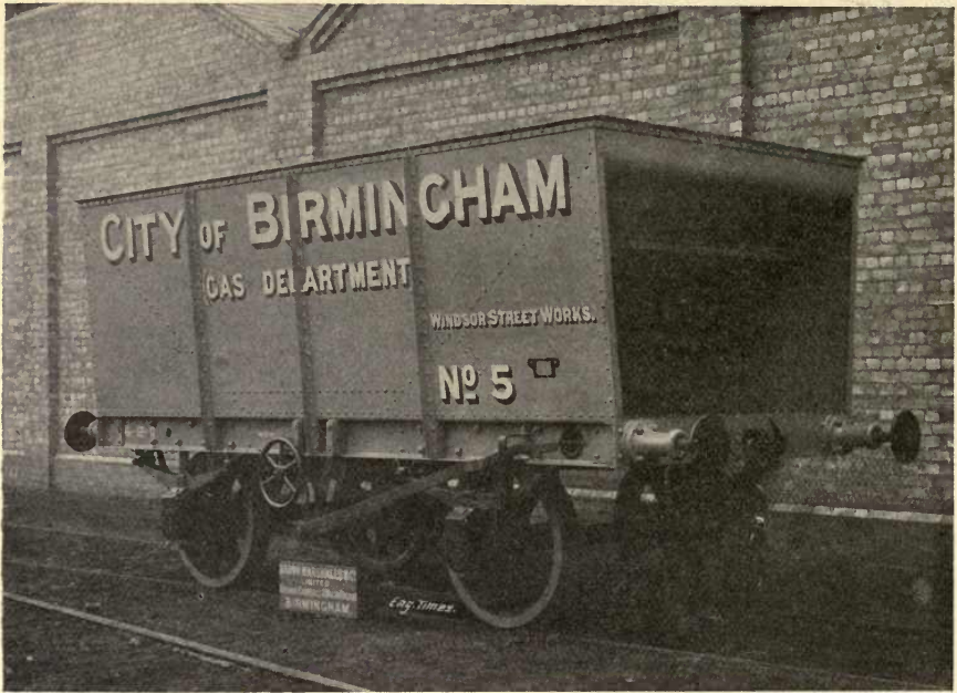
FIG. 5.—AUTOMATIC HOPPER WAGON.
