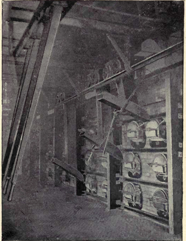
FIG. 16.—VIEW OF TRAVELLING SHOOTS AND OPERATING LEVERS ON CHARGING STAGE.
