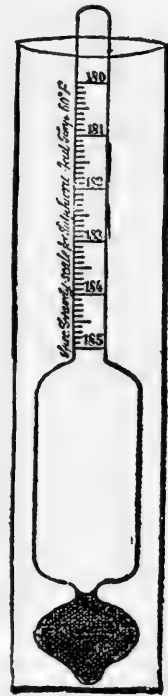
FIG. 18 HYDROMETER FOR TESTING STRENGTH OF SULPHURIC ACID
