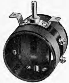
Fig. 6 Two Inductances with variable coupling.
