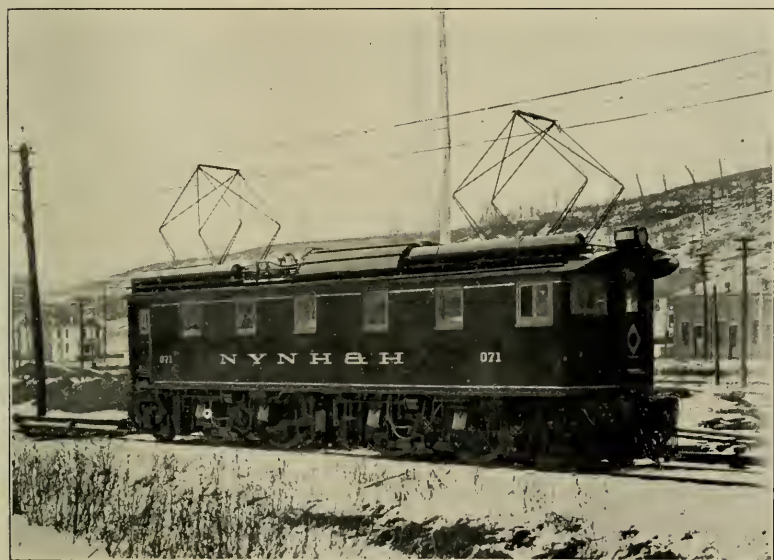
HEAVY SERVICE, ALTERNATING AND DIRECT CURRENT FREIGHT LOCOMOTIVE BUILT BY THE WESTINGHOUSE COMPANY FOR THE NEW YORK, NEW HAVEN & HARTFORD RAILROAD
