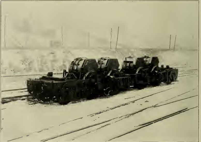
THE OUTER SHELL OF THE NEW HAVEN'S FREIGHT LOCOMOTIVE REMOVED, SHOWING THE WORKING PARTS OF THE MACHINE
