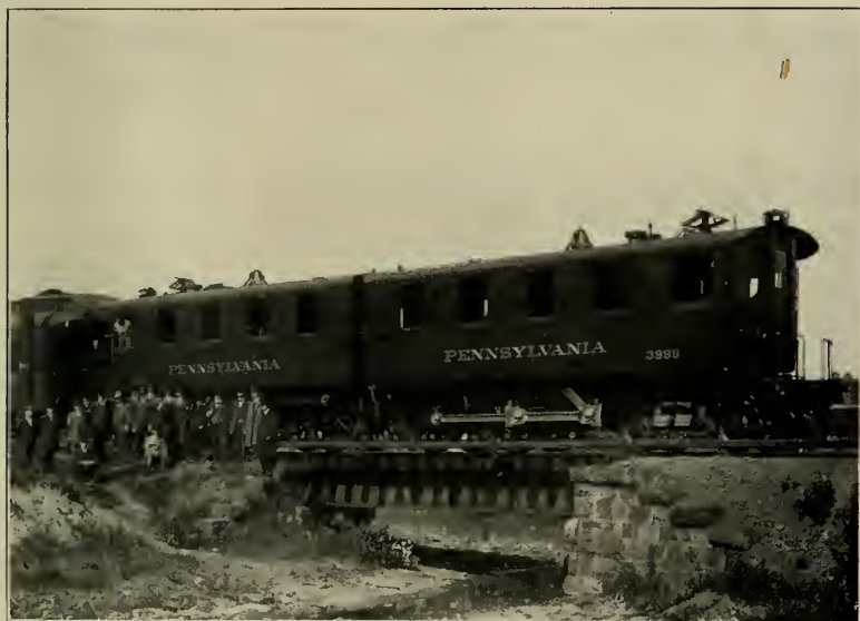
HIGH-SPEED DIRECT-CURRENT LOCOMOTIVE BUILT BY THE WESTINGHOUSE COMPANY FOR THE TERMINAL SERVICE OF THE PENNSYLVANIA RAILROAD, IN NEW YORK
