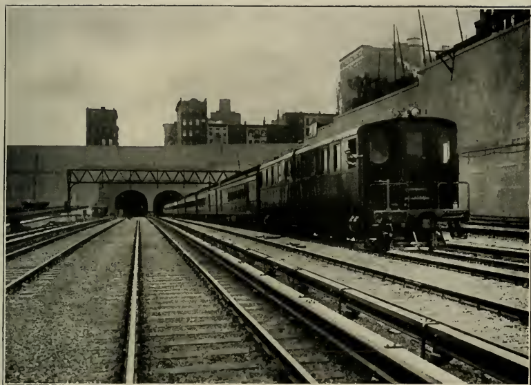
A HIGH-SPEED ELECTRIC LOCOMOTIVE ON THE PENNSYLVANIA BRINGING A THROUGH TRAIN OUT OF THE TUNNEL UNDERNEATH THE HUDSON RIVER AND INTO THE NEW YORK CITY TERMINAL
