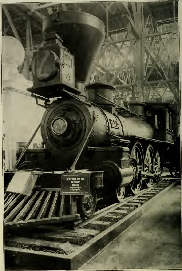
A HEAVY-GRADE TYPE OF LOCOMOTIVE BUILT FOR THE BALTIMORE & OHIO RAILROAD IN 1864. ITS FLARING STACK WAS TYPICAL OF THOSE YEARS
