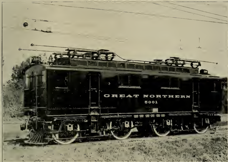
TRIPLE-PHASE ALTERNATING-CURRENT LOCOMOTIVE BUILT BY THE GENERAL ELECTRIC CO. FOR USE IN THE CASCADE TUNNEL, OF THE GREAT NORTHERN RAILWAY
