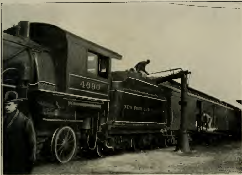
“ WHEN THE TRAIN COMES TO A WATER STATION THE FIREMAN GETS OUT AND FILLS THE TANK ”
