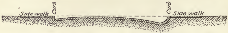
Fig. 76. Street with Unequal Transverse Grade Inclined so as to Drain by Lower Gutter
