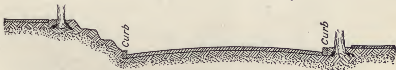
Fig. 75. Street with Unequal Transverse Grade but with Level Street
