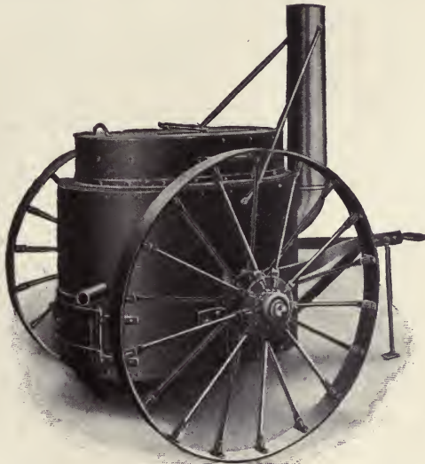
Fig. 88. Coal-Tar Heating Tank Courtesy of Barber Asphalt Paving Company, Philadelphia, Pennsylvania
