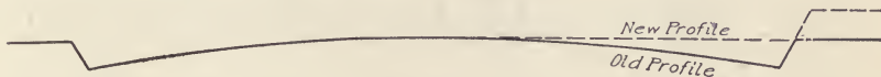
FIG. 14. Diagram Showing Adjustment of Profile on Curves for Rapidly Moving Motor Vehicles
