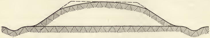
Fig. 32. Section Showing Correct Slopes of Embankments
