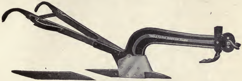
Fig. 43. Typical Hardpan or Rooter Plow Courtesy Western Wheeled Scraper Company, Aurora, Illinois
