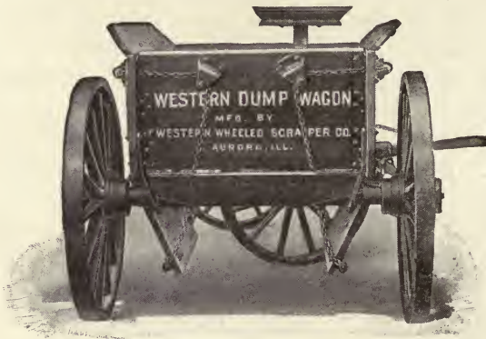
Fig. 50. Rear View of Typical Dump Wagon Showing Bottom Open Courtesy of Western Wheeled Scraper Company, Aurora, Illinois
