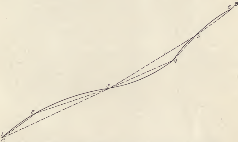
Fig. 6. Diagram Showing Method of Approximating Elevation of Successive Contours of Inclined Road
