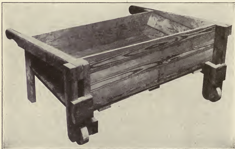
Fig. 86. Grout Box Used in Laying Brick Pavement Courtesy of National Paving Brick Manufacturers Association, Cleveland, Ohio
