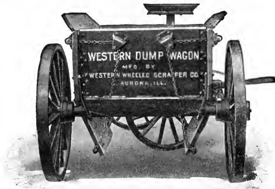
Fig. 50. Rear View of Typical Dump Wagon Showing Bottom Open Courtesy of Western Wheeled Scraper Company, Aurora, Illinois
