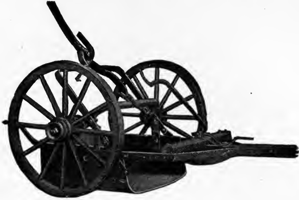
Fig. 46. Typical Wheeled Scraper Courtesy Western Wheeled Scraper Company, Aurora, Illinois
