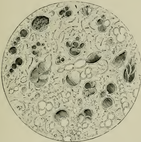
FIG. 34.—SECTION OF BITUMINOUS LIMESTONE of Neby Mousa, magnified, showing, Globigerina , Textularia , etc., with the cavities of some of them filled with bitumen, which also saturates the intervening matrix, composed of Coccoliths and fragments of Foraminifera.
