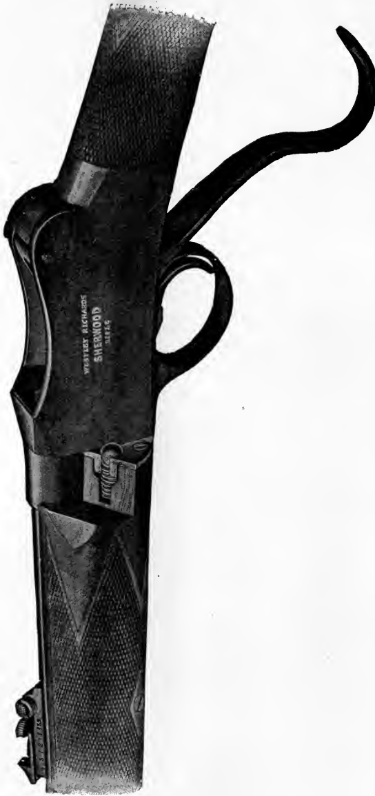
FIG. 184.—THE WESTLEY RICHARDS DETACHABLE BARREL, WITH PATENT LOCKING LUGS, IS SECURED IN POSITION BY THE METHOD ILLUSTRATED. At the end of the fore-end is shown the steel ball or boss, which rides upon a spiral spring; on turning the barrel about a quarter turn the steel boss is pressed within.
