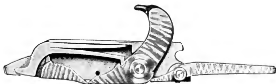
FIG. 24.—THE WESTLEY RICHARDS HAND-DETACHABLE LOCK.
