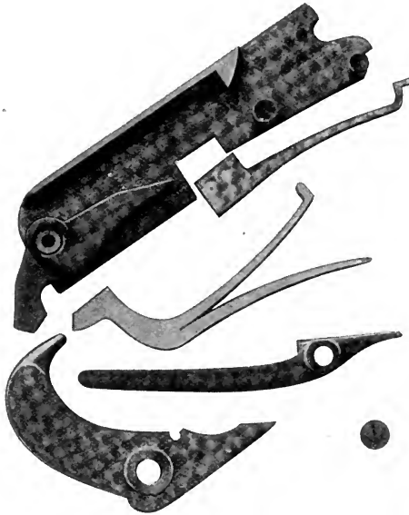
FIG. 26.—THE 7 PARTS OF THE WESTLEY RICHARDS (A. AND D.) LOCK.
