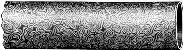
FIG. 5.—BOSTON OR TWO-STRIPE DAMASCUS BARREL.
