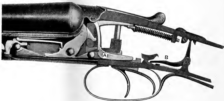
FIG. 30.—TUMBLER SAFETY BOLT OR SECONDARY SEAR AND TRIGGER SAFETY.
