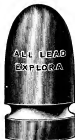
FIG. 99.—WESTLEY RICHARDS LEAD-CAPPED BULLET.
