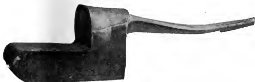
FIG. 11.—ROUGH FORGING OF ACTION-BODY.
