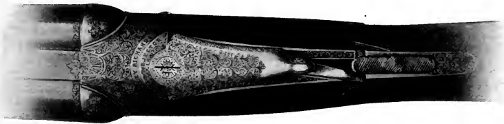
FIG. 81.—SHOWING STOP MOVED ASIDE AND THE SAFETY SLIDE PUSHED FORWARD FROM THE SAFE POSITION.
