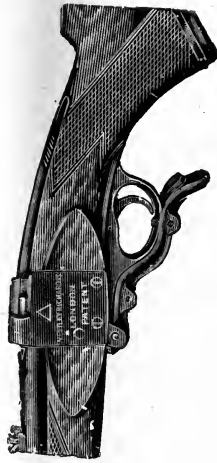
FIG. 179.—UNDER-LEVER SLIDING-BLOCK ACTION.
