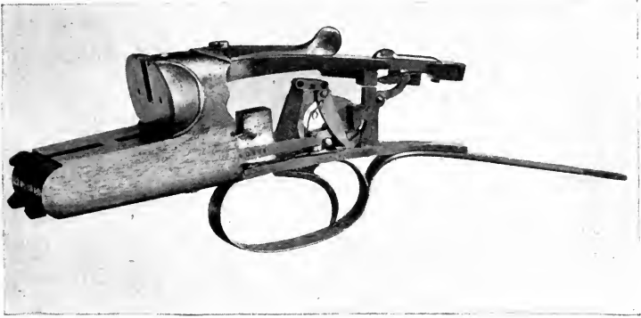
FIG. 12.—ACTION-BODY COMPLETE IN THE FILED STATE.
