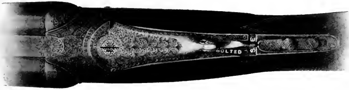
FIG. 80.—SHOWING STOP BOLTING THE SAFETY SLIDE. THIS PREVENTS THE SLIDE FROM BEING ACCIDENTALLY MOVED FROM THE SAFETY POSITION.
