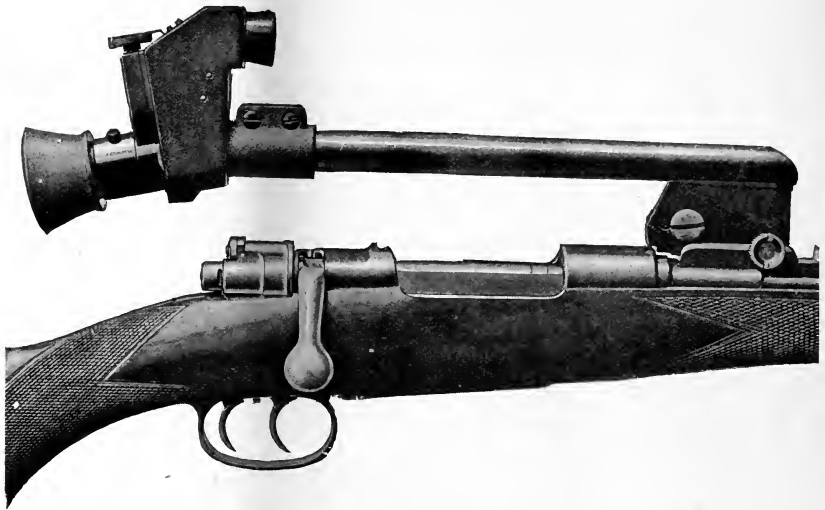
FIG. 150.—ZEISS TELESCOPE SIGHT WITH WESTLEY RICHARDS ATTACHMENT.
