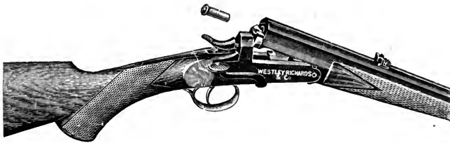
FIG. 177.—SIDE-LEVER ACTION, REBOUNGING LOCK.
