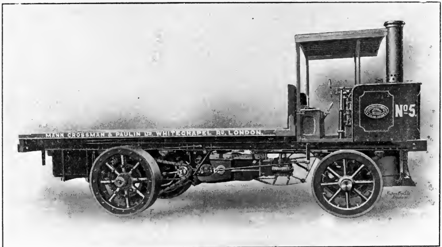
Fig. 43. Lancashire Steam Motor Co. 4-Ton Wagon.
