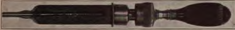
FIG. 13.—Handle of Bigelow's lithotrite, showing locking mechanism by which the blades are locked upon the stone or released from it.
