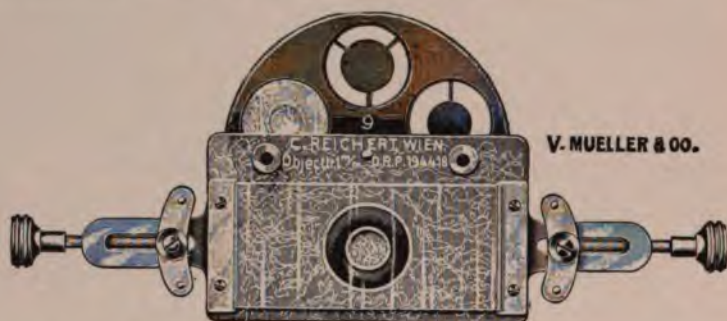
FIG. 140.—The Reichert apparatus for "dark-ground" illumination, to be attached to the microscope stage.
