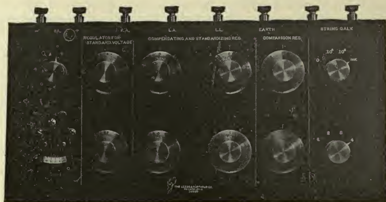
Fig. 215.—The Williams-Hindle Electrocardiographic Outfit. (By courtesy of Dr. H. B. Williams.)
