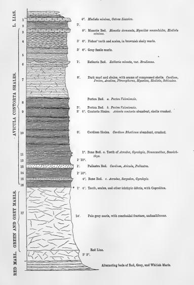
FIG. 2.- A Vertical Profile of Aust Cliff.
