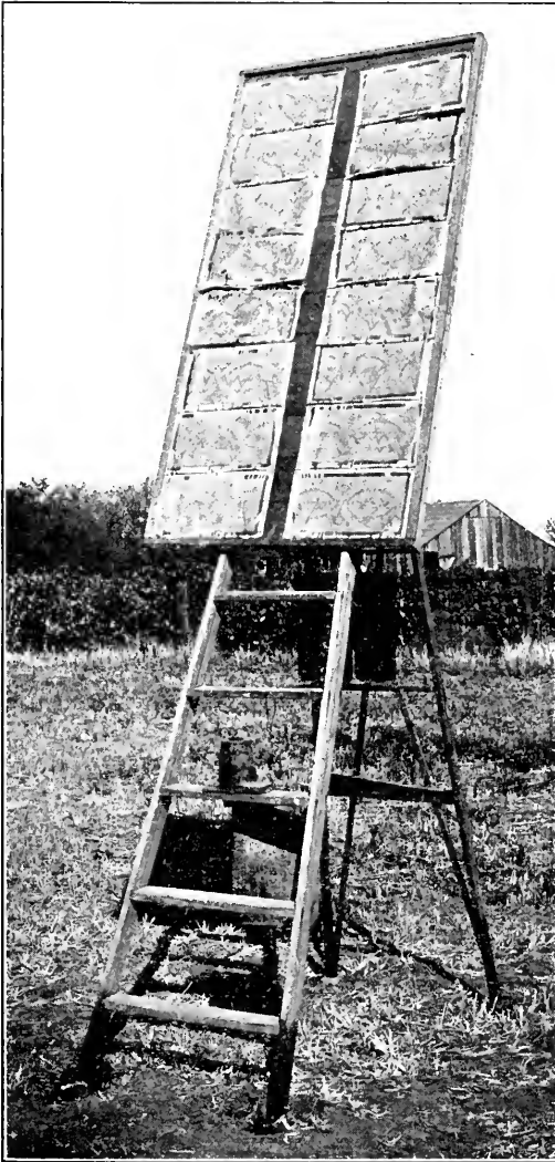
FIG. 407.—Close view of the apparatus showing the legs standing in cans of water and oil. (Photo by Geo. P. Weldon.)
