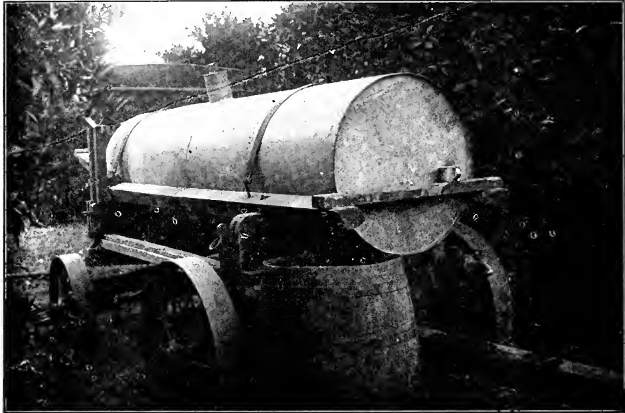
FIG. 315.—A water supply wagon for a large fumigating outfit. (After Pierce, P. C. Jr. Ent.)
