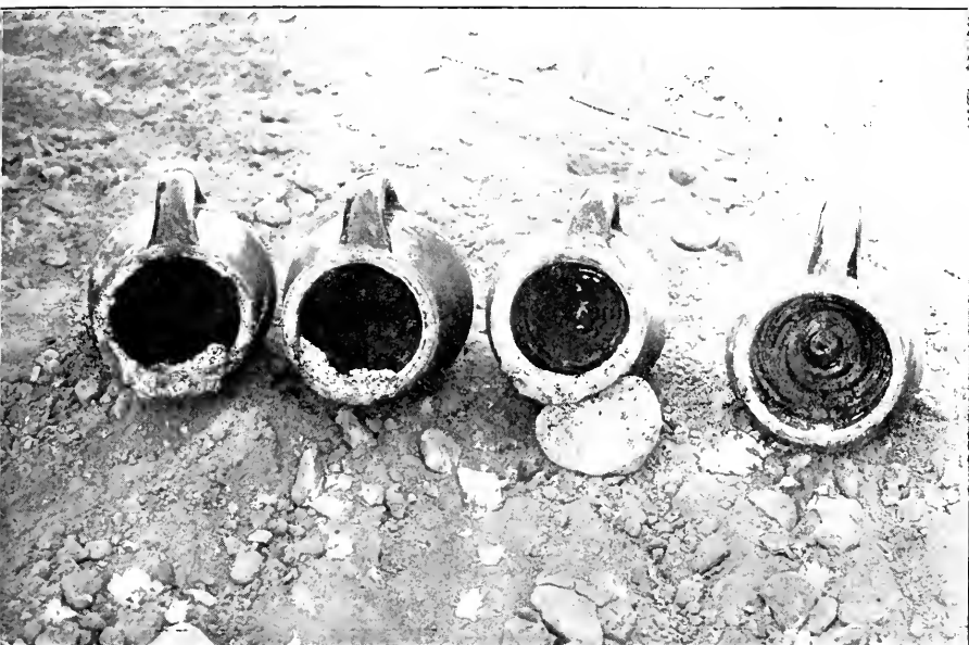
FIG. 314.—Acid generators showing residue remaining because of careless emptying. (After Pierce, P. C. Jr. Ent.)
