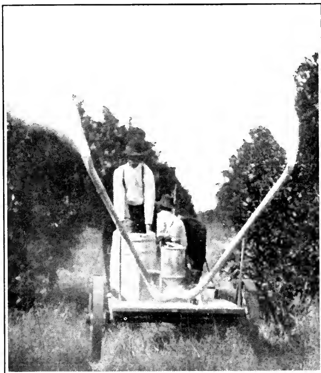
FIG. 304.—A power blower for applying dust sprays in orchards. About forty acres can be treated in one day with such a machine. It costs $115.00.
