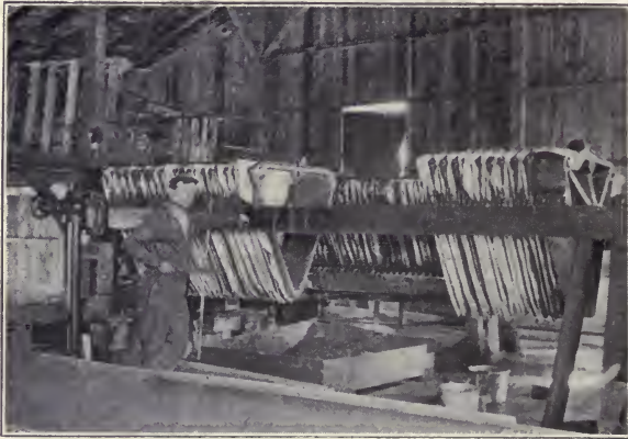
Fig. 41. ZINC-DUST PRECIPITATION PRESSES Showing part of cake in place at time of clean-up
