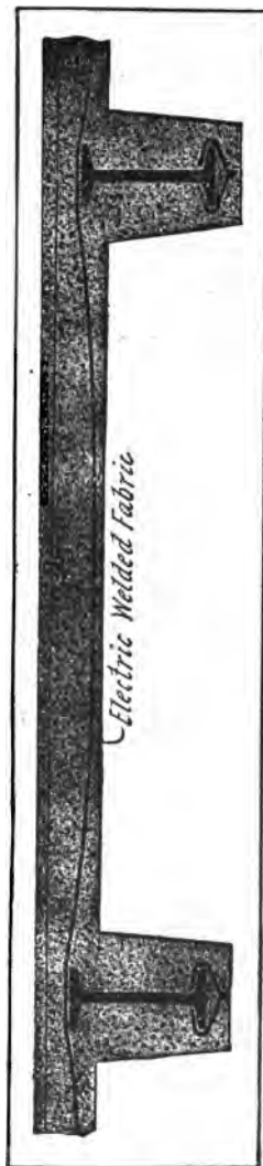
Fig. 11.—Clinton System Using Electrically Welded Fabric.
