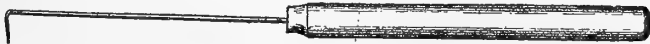
FIG. 16.—Setting needle used in adjusting wings of micro-lepidoptera upon the glass surface of the setting board.
