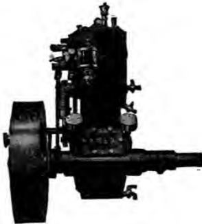
Knox Single-Cylinder, 2-cycle, 3-port Engine.
