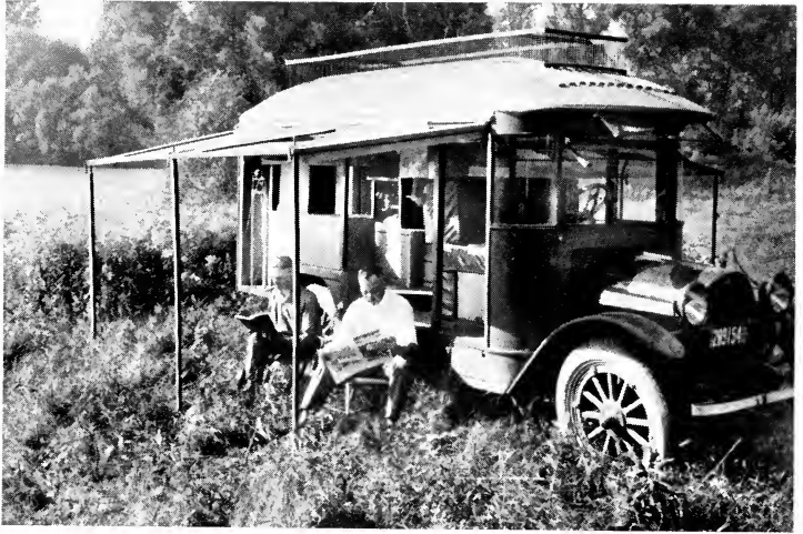
Specially built touring bungalow, on a Reo chassis, adapting the Pullman idea to the motor vehicle
