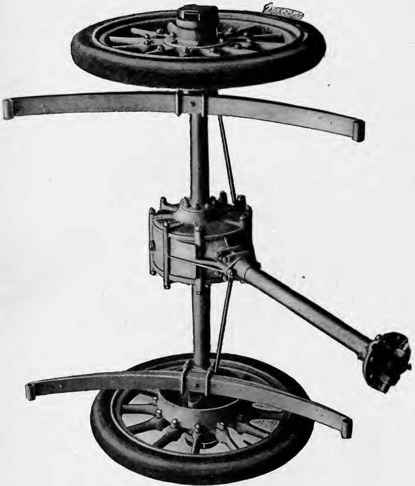
FIG. 31.—Live Axle with Encased Shafts.
