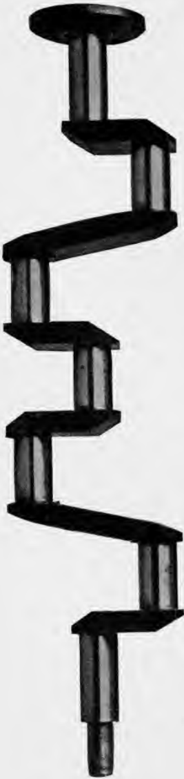
FIG. 25.—Crankshaft for Small Four-Cylinder Engine. This has only three main bearings.
