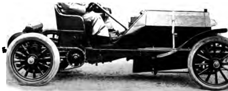
LANCIA ON F.I.A.T. RACER, 1905, ON WHICH HE COVERED 198 MILES AVERAGE SPEED OF 69.9 MILES PER HOUR Wheelbase, 10 ft.
