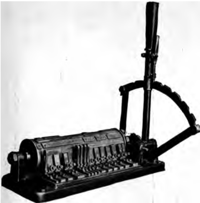
Fig. 2.—A controller for an electric car
