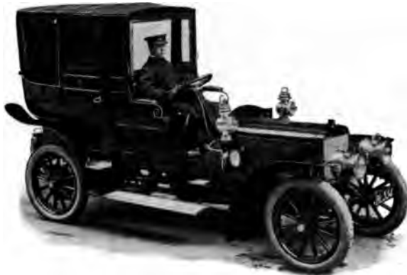
H. R. H. Princess Christian's 24 h.-p. Thornycroft Landauet Extreme length, 14 ft. 6 in.
