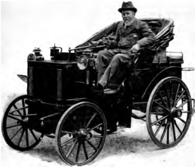
The first Petrol Car introduced into England—the Hon. Evelyn Ellis's 4 h.-p. Panhard and Levassor Car
