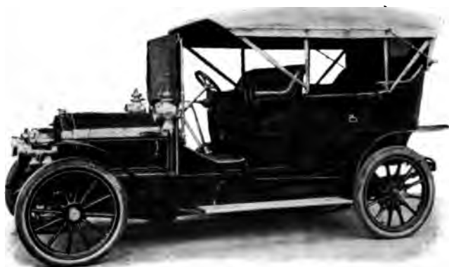
15 h.-p. Siddeley, with live axle and direct drive Extreme length, 13 ft.
