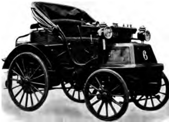
PANHARD ET LEVASSOR, 1896 4 CYLINDERS PARIS-MARSEILLES TYPE Average speed, 15.6 miles per hour
