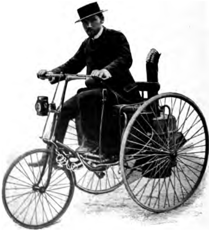
Mr. Snow's first steam bicycle (coal-fired) (date 1887)
