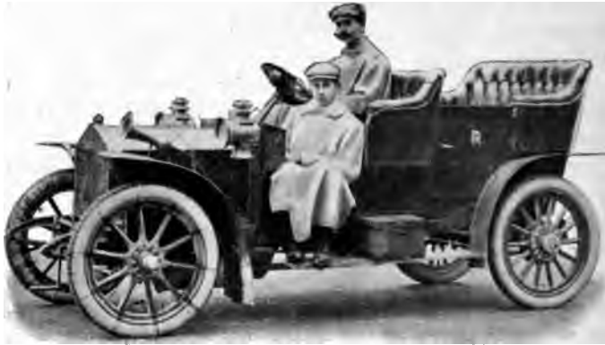
Rolls-Royce Tourist Trophy Car, 1905. Ran second. 208½ miles, at a speed of 33½ miles per hour. Fuel consumption one gallon for 24·8 miles (Driven by Mr. Percy Northey, an amateur)
