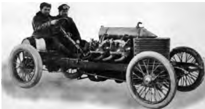
(Photo by M. Branger, Paris) THE 8-CYLINDER DARRACQ, 1906. SPEED 122½ MILES PER HOUR Wheelbase, 7 ft. 11 in. (Supplied by the Topical Press Agency)
