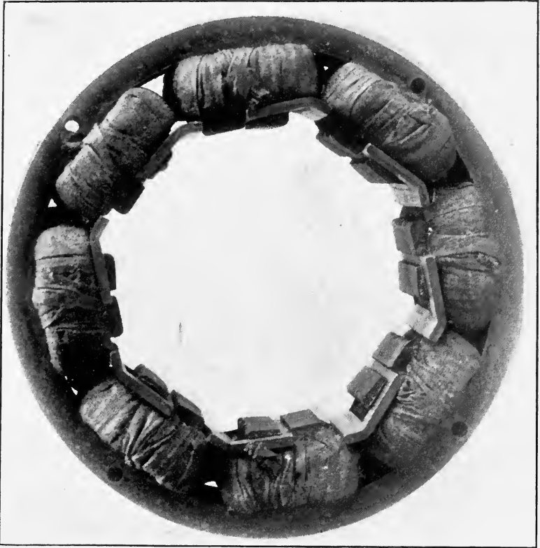
Fig. 157.—Single-phase stator, showing shading-coils.
