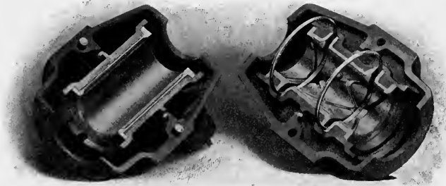
Fig. 31.—Bearing housing open, showing bearings, oil wells, and oil rings. Westinghouse Co.
