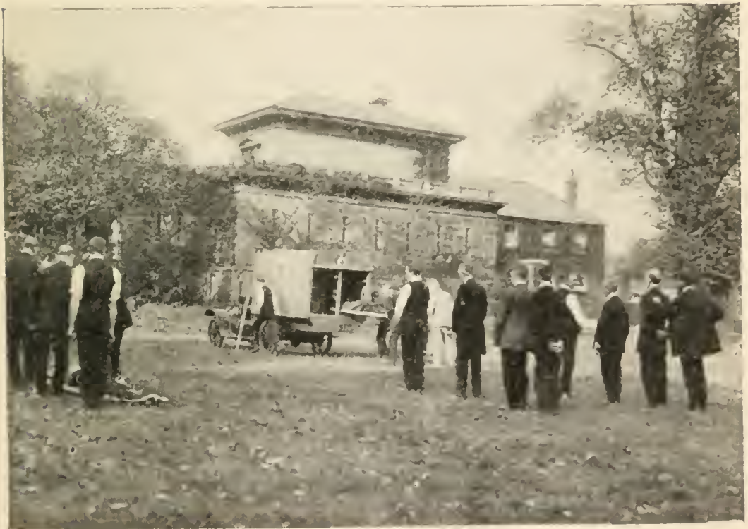
LOADING THE STRETCHER INTO THE CAR BODY. IT IS AFTER- WARDS RAISED FORE AND AFT AND ATTACHED BY STRAPS TO THE SPRING HOOKS PROVIDED. NOTE THE MEN RUNNING TO THE FRONT TO LIFT THE FORWARD HANDLES.
