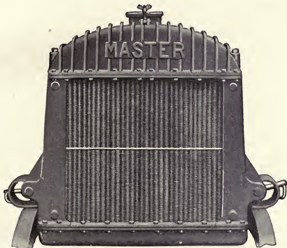
FIG. 37. Flat Spiral Spring Mounting of the Master Trucks.
