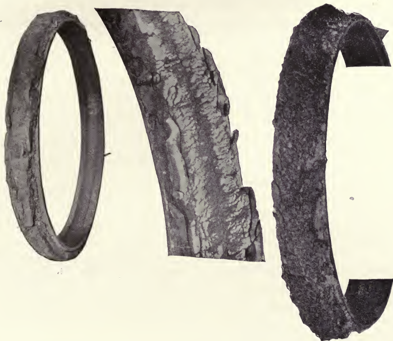
FIG. 278. Overloaded, Overspeeded and Bad Road Tire Effects.
