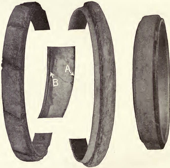
FIG. 282. Tires Showing Undue Wear.
