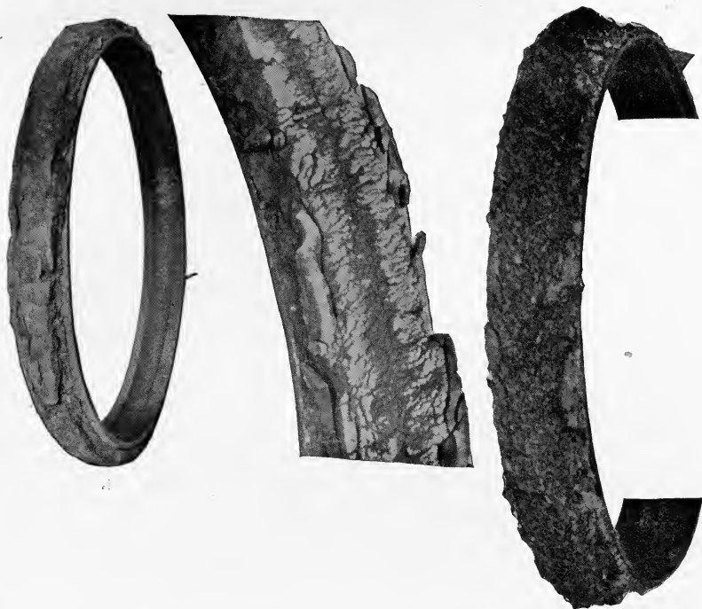
FIG. 278. Overloaded, Overspeeded and Bad Road Tire Effects.
