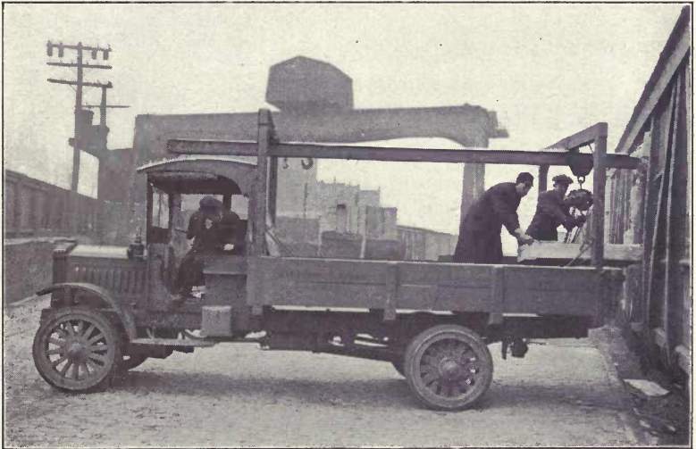
The overhead loading track and chain hoist with which this truck is equipped simplifies loading the truck with heavy materials.
