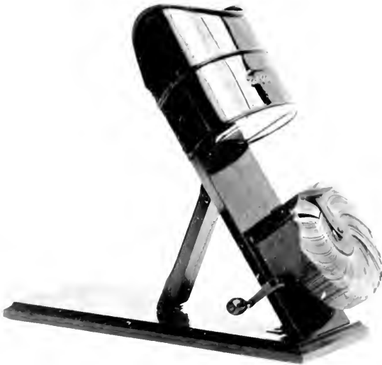
The Kinora reproduction instrument. It resembles a stereoscope, and the pictures are exposed singly by rotating the handle.
