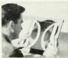
Castings are placed around the Bomb, with a sensitive film behind each. Bomb's rays pass through casting, giving a "photo" of the inner structure of the metal.
