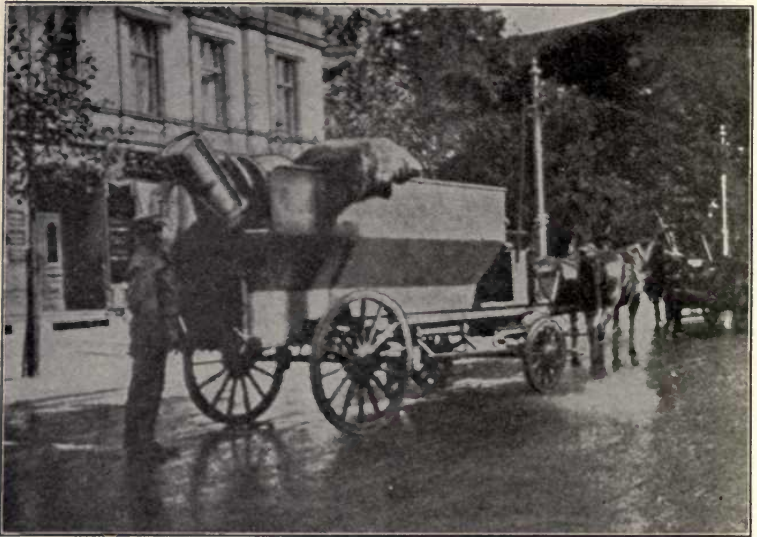
FIG. 138.—CHARLOTTENBURG, NEAR BERLIN. HOUSE REFUSE CART WITH CAN OF REFUSE BEING EMPTIED BY A MECHANICAL APPLIANCE WHICH PREVENTS THE ESCAPE OF DUST AND ODOR.
