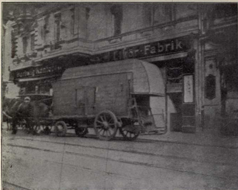
FIG. 139.—COVERED WOODEN CART USED IN BERLIN, GERMANY, TO COLLECT HOUSE REFUSE. THIS CART IS INTENDED TO BE DUSTLESS AND ODORLESS. (Courtesy of Dr. Soper.)
