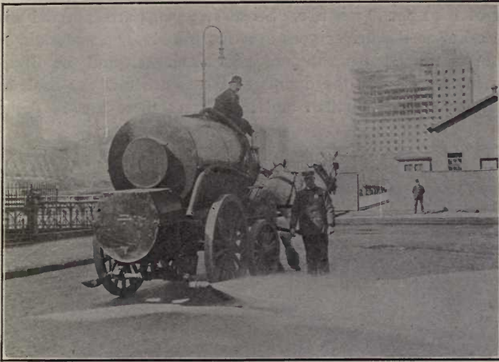
FIG. 146.—STUDEBAKER FLUSHING MACHINE WITH GASOLINE ENGINE AND PUMP.
