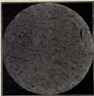
FIG. 225.—FORMULA 8, ATLANTIC CITY TEST FENCE; COMBINATION TYPE AFTER FIFTEEN MONTHS.
