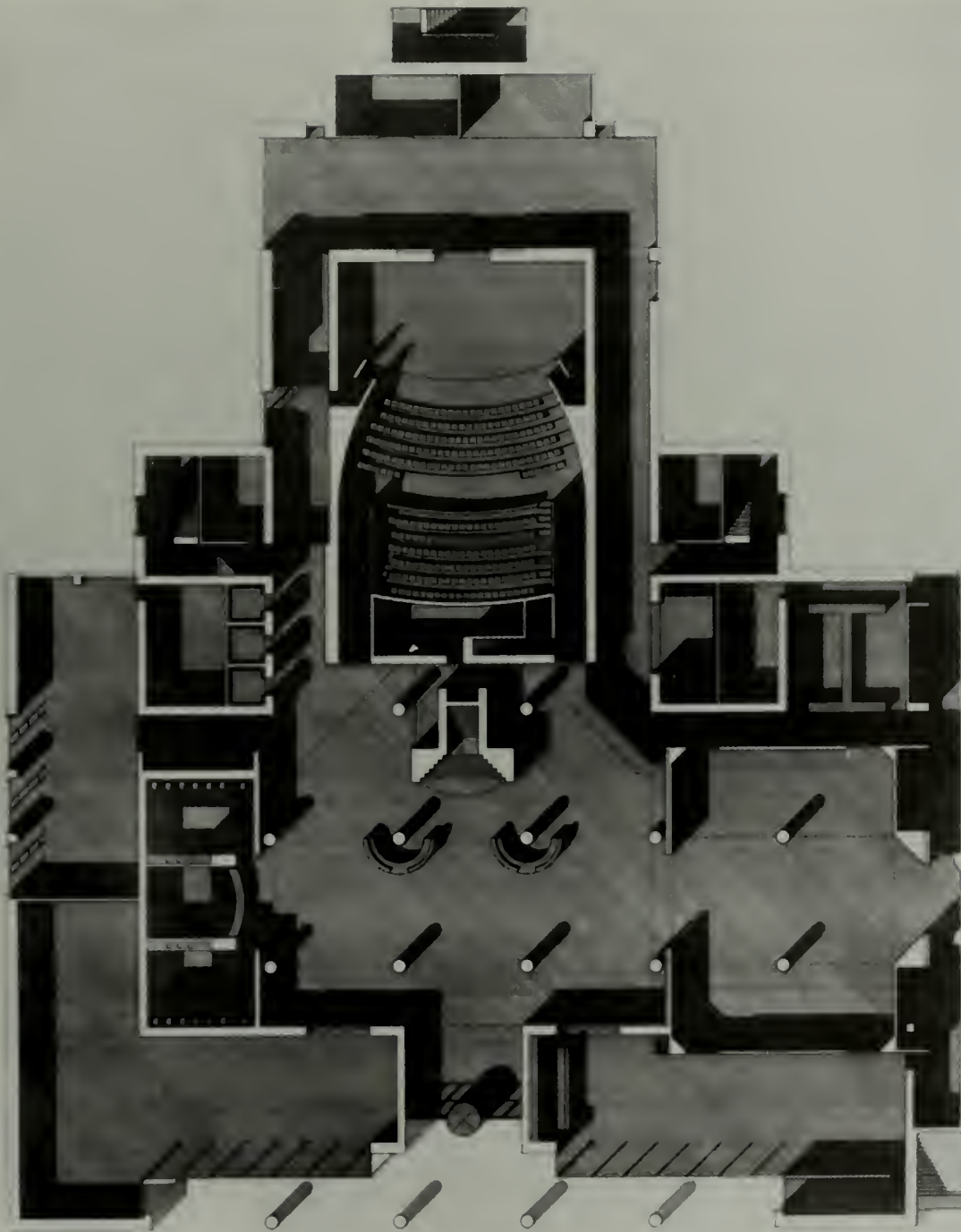
San Francisco Museum of Modern Art (Mario Botta, 1990). These four illustrations show the cumulative benefit derived from a basic ground-floor plan (a); then a longitudinal section (b), which enables the viewer to see through the building at all levels; followed by façade-elevation renderings (c and d), which give only single points of view but which detail significant façade features, like the central cylinder. (Photos: Ben Blackwell)
