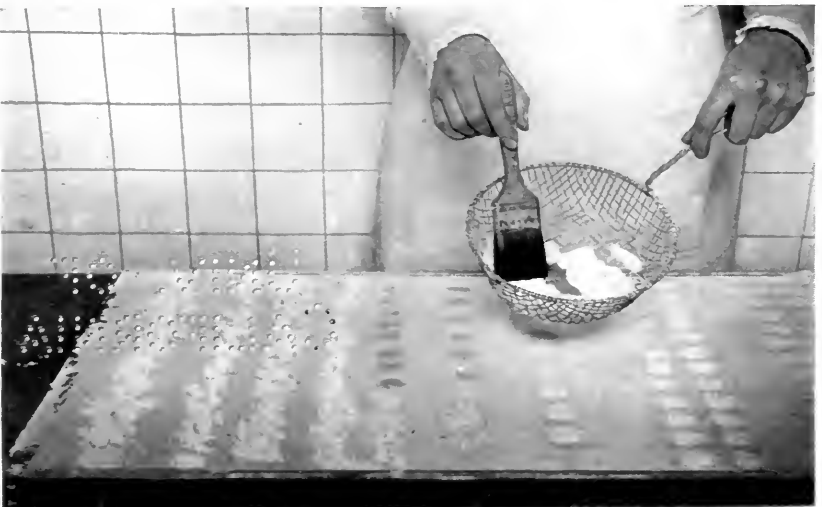
Removing Starch from hardened Creams by Brushing
