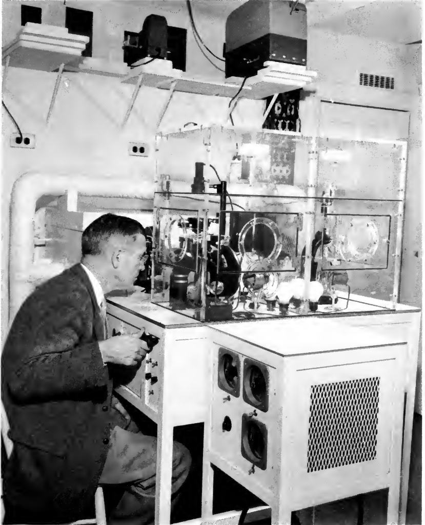
Latest improved microscopic time-lapse unit with all microscope controls extended outside of plastic cabinet. In background is special heating and refrigeration unit for controlling the temperature of the microscope stage and subject being photographed. Smaller cabinet in foreground contains all automatic timing equipment that might jar or move subject being photographed in microscope.
