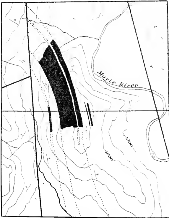
Figure 13. Locality map of the Moyie sills, showing in solid black the parts best exposed. The straight line in the middle of the map represents the Boundary line; the other straight lines represent the approximate outcrops of major faults. The block between the faults includes Moyie mountain. Contour interval is 500 feet. Scale, 1 : 68,000.
