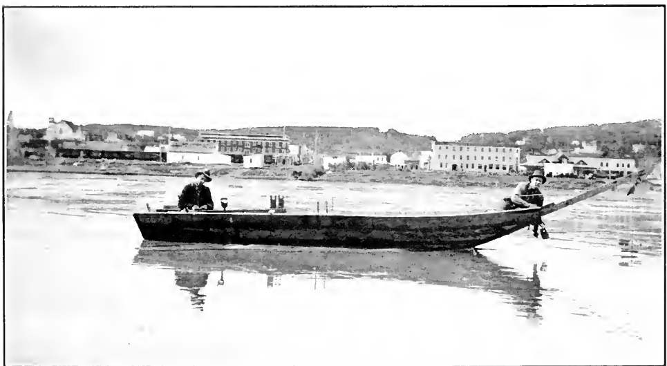
Boat used for making Discharge Measurements of Athabaska River at Athabaska, Alberta. Taken by G. H. Whyte.
