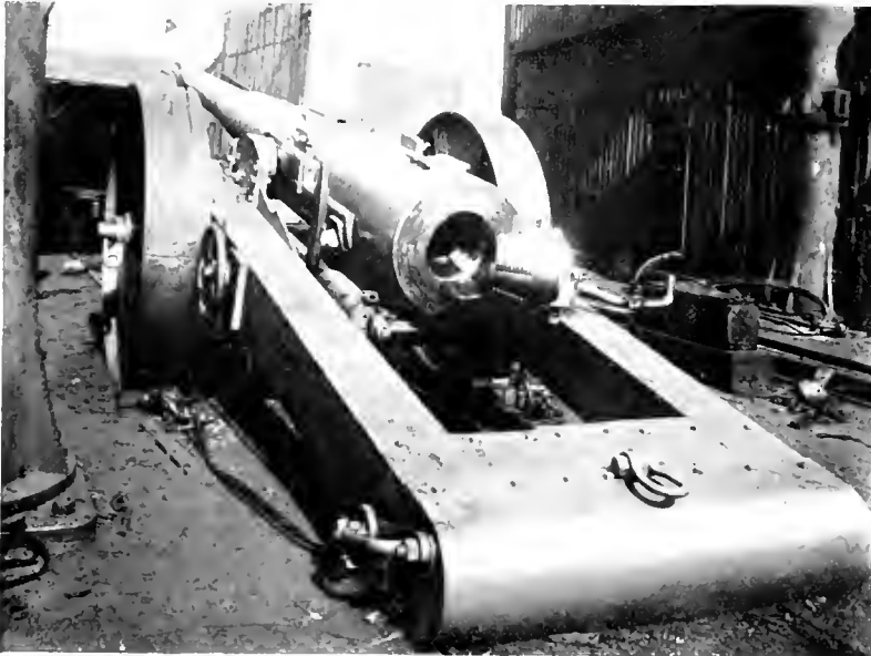
CARRIAGE OF 100-LB. GUN CONSTRUCTED IN N.G.R. LOCO. SHOPS
