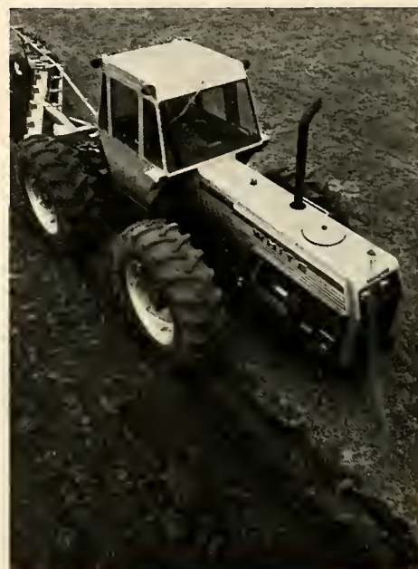
White Farm Equipment's new "Field Boss" four-wheel drive row crop tractor features a Caterpillar V8 engine and low profile design for powerful pulling and maneuverability.
